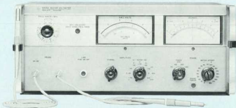
Fig. 1. -hp- Model 8405A Vector Voltmeter measures amplitudes and phase simultaneously. Instrument has frequency range of 1 MHz to 1 GHz, sensitivity of 100 \mu V full-scale, dynamic range of 95 dB, phase resolution of 0.1°, and is simple to operate. Thus it makes feasible many measurements which formerly were difficult or impossible.
